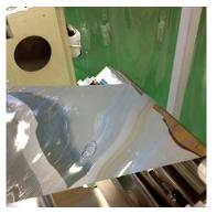
TDC developed a special machine just for long foils. It continuously supplies foil to the lapping machine to polish. After the polishing, it automatically rolls it up again.
