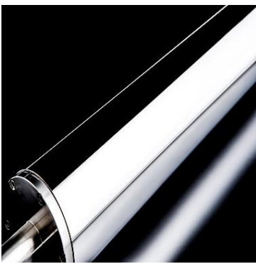
Super precision polished Roll Applied to high spec film, Nanoimprinting technology. Max : dia.450*L3,000 mm Ra1.5 nm, Rz8 nm (Stainless steel)
