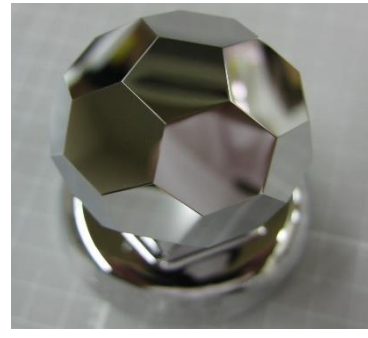
Other shapes We have many special lapping machines for polishing not only flat items but curves, Inner diameter of cylindrical shape, spherical bodies. Their polishing will also be finished in Ra1 nm level.
